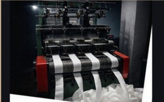
Precision weaving process for high-strength nylon 66 curing tape
